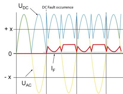
Illustration 3: Insulation fault causing DC current
