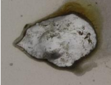
Soldering test showing good surface wetting
