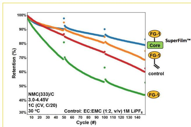
**Figure 2:** Modular electrolyte additive with core species and functional group gives best capacity retention during high voltage cycling
