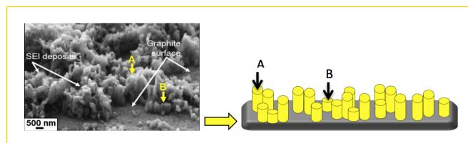
**Figure 1:** SEM of graphite showing non-uniformity of SEI layer
