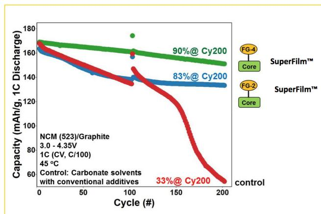
**Figure 5:** Wildcat modular electrolyte additives show significant cycle life improvement for NCM (523) at elevated temperature and voltage
