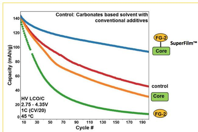
**Figure 3:** Modular electrolyte additive with core species and functional group gives best capacity retention at during elevated temperature cycling
